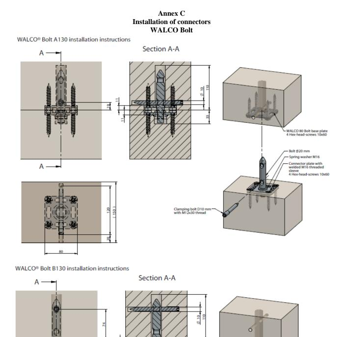
Clamping bolt D10 m with M12x30 thread Bolt Ø20 mm Spring washer M16 Connector plate with welded M16 threaded sleeve 4 Hex-head-screws 10x60
