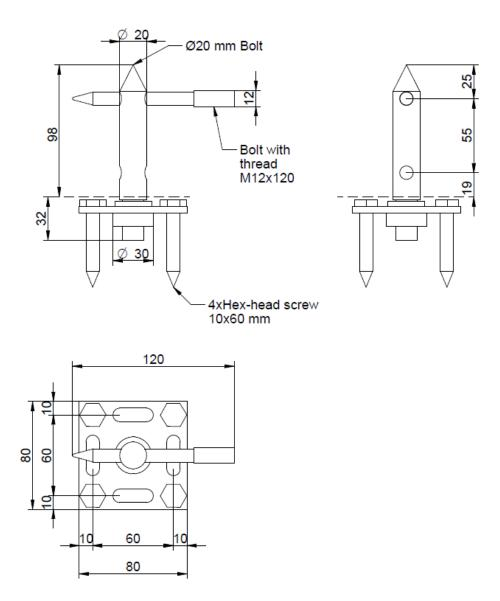
4 screws per plate, with KNAPP® WALCO® V PH screw 10x60
