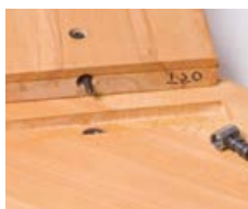
Insert clamping elements in holes
