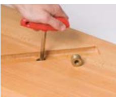
Screw-in threaded insert (SW 10)
